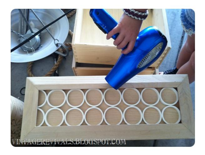
The PVC fit so perfectly and tight in the fronts that we did not glue every single circle. We just put glue in a few spots to make sure that it stayed in place.
