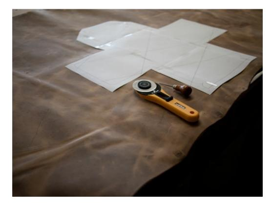
Before starting, print out the template on your printer using the "tile" function and tape it together to 100% scale. The one shown in the pic was an earlier version before I decided to cut the flaps separately. You can cut this from one piece of leather, but there's more waste with the voids than with making separate flaps. If you modify this for your own project, maybe it's smart to use one piece? That's where this experiment can get really fun.
