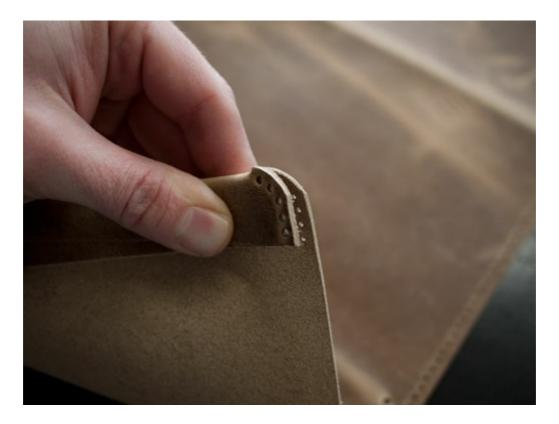
5. The final step is to hand-sew your pieces with two needles and thick waxed thread. Using the two-needle method and backstitching on your ends will give you a sturdy, long-lasting seam. Again, there are more in-depth stitching lessons on my passport post.
